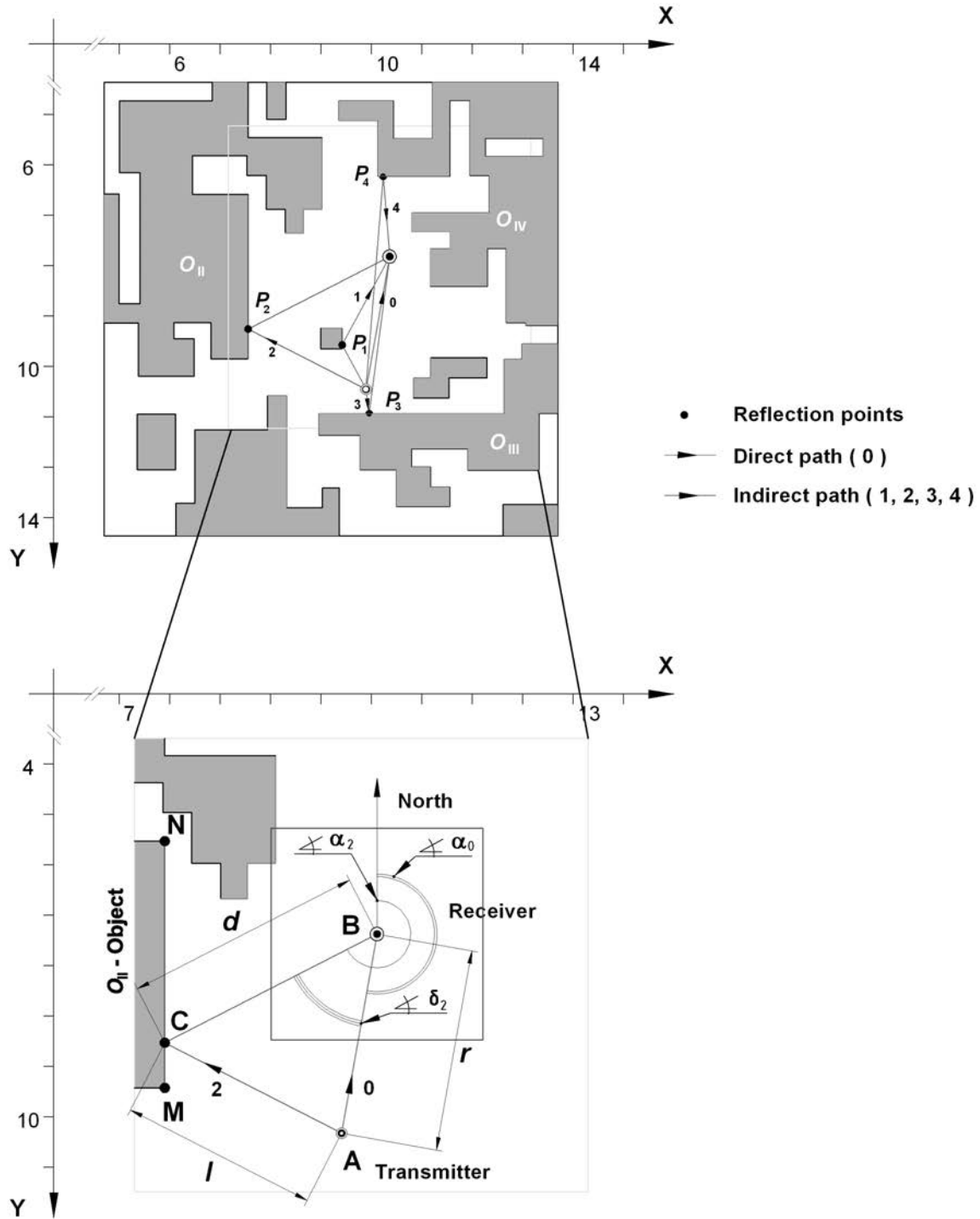
Figure 2: The upper part shows a digital map with a-priori known objects and relevant propagation paths based on single reflections. The lower part shows an extract of the above figure tailored to the reflection path 2, together with definition of angles and lengths relevant for the hybrid algorithm
