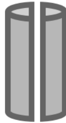
Figure 12 Example of different description of the same geometry Default interpretation of a hole from Creo to STEP, which contains two cylindrical surfaces
